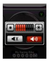
Figure 7. Brightness and volume controls
