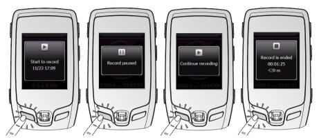
Figure 10. Recording with the side control button
